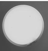
CONNECTOR END (PROXIMAL END) AFTER USE AND STILL NO DAMAGE VISUABLE
